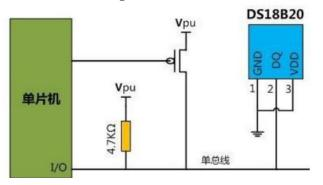
Figure 1. Hardware connection diagram.
