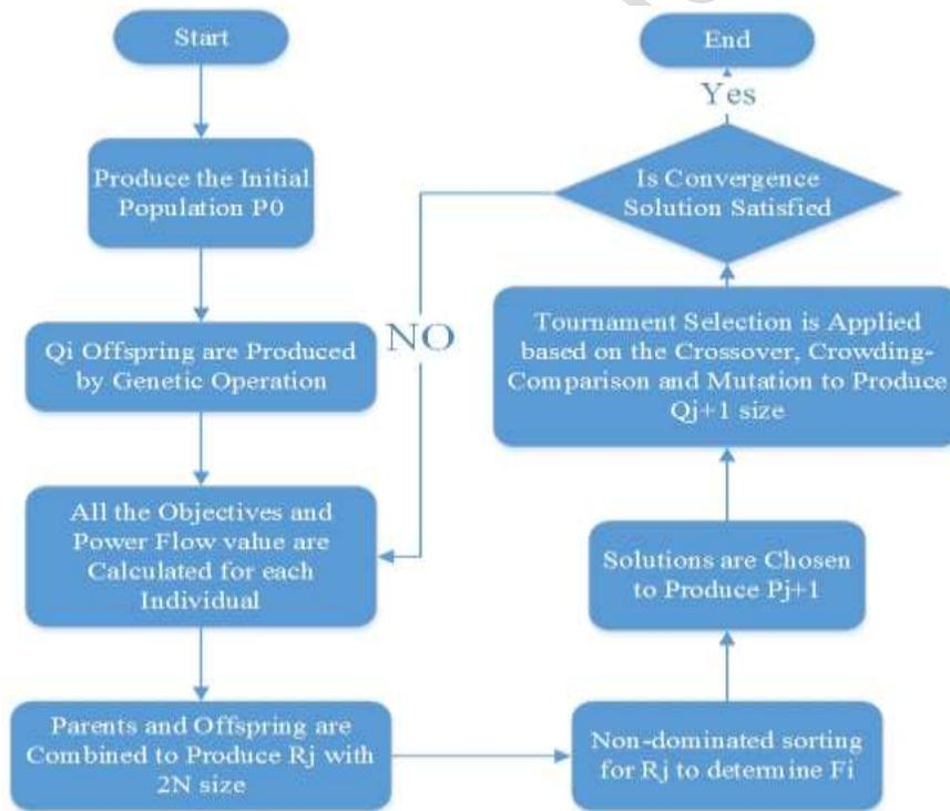
Figure 5. Flow chart of NSGA-II solving process.
