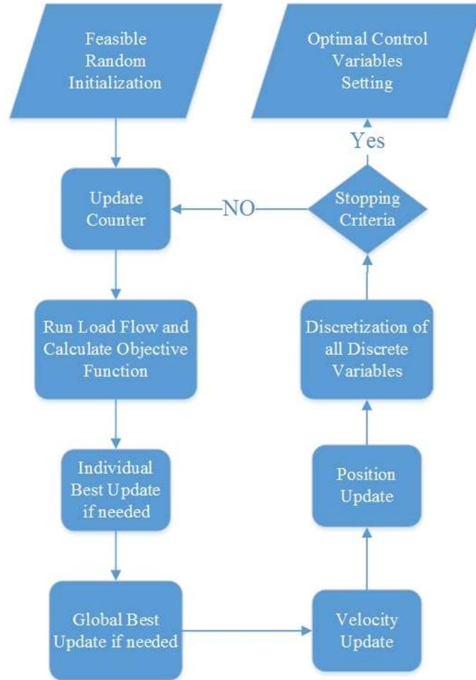
Figure 7. Single objective OPF algorithm using PSO algorithm
