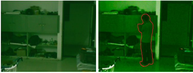
Fig. 5. (a) Room monitoring with motion sensors and camera, (b) Intruder detected by system
