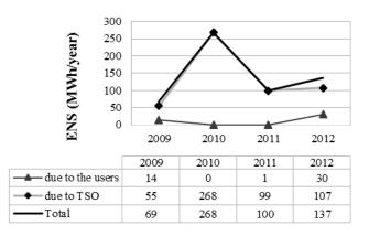
Figure 1. The Energy Not Supplied (ENS) per year. (data processed from website: http://www.transelectrica.ro)
