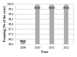
Figure 4. Framing duration of frequency within the normal range of variation: (49.90-50.10) Hz. (data processed from website: http://www.transelectrica.ro)
