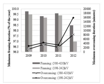
Figure 5. Overcoming the admissible voltage range on voltage levels (220 kV si 400 kV). (data processed from website: http://www.transelectrica.ro)
