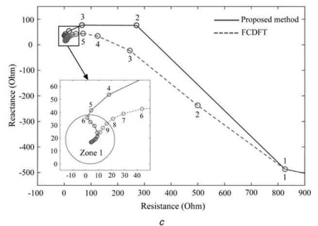
**Fig. 11** Trajectories of the measured impedances for the real data test cases
