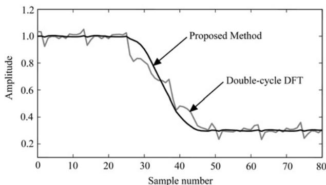
**Fig. 3** Estimated phasor amplitudes using the proposed and the conventional double-cycle fourier algorithms for a frequency drift case
