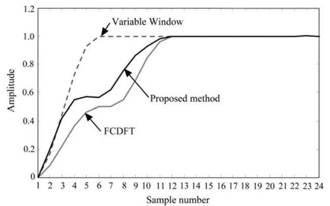
**Fig. 4** Estimated phasor amplitude using the proposed, FCDFT and variable-window algorithms for a pure sinusoidal signal, case I
