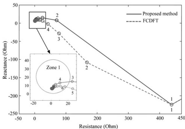
**Fig. 9** Trajectories of the measured impedance for the A-G internal fault
