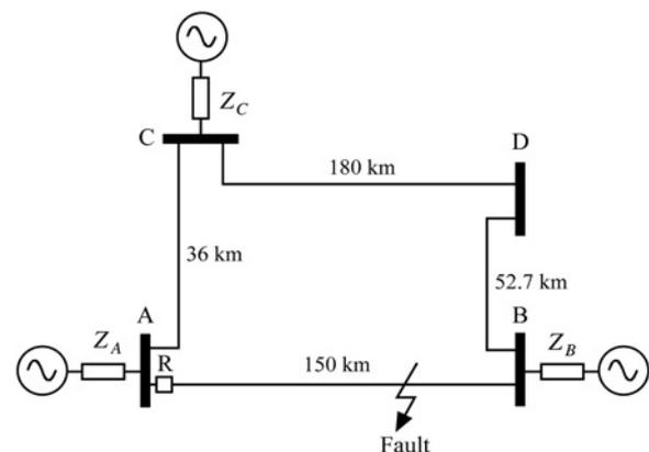
Fig. 8 Model of the simulated transmission system
