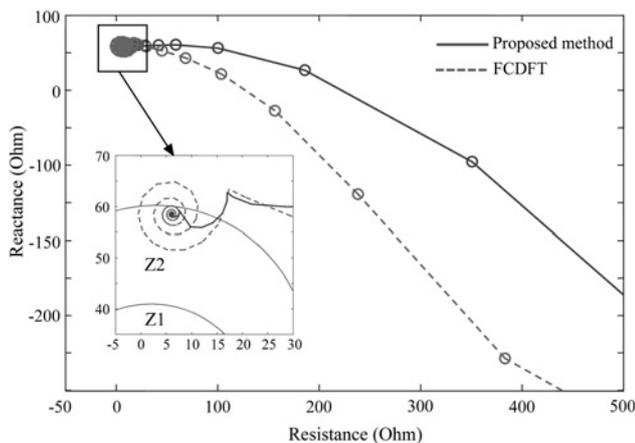
**Fig. 10** Trajectories of the measured impedance for the A-B-G external fault
