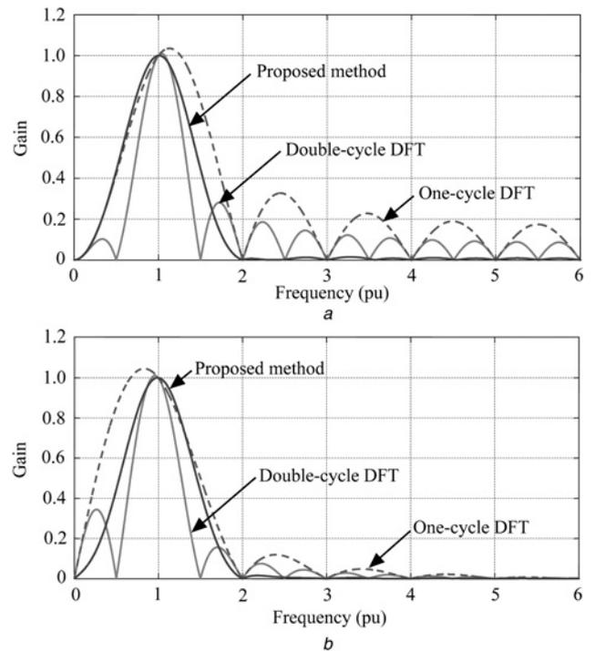
**Fig. 2** Frequency responses of the proposed digital filters, one-cycle and double-cycle Fourier filters
