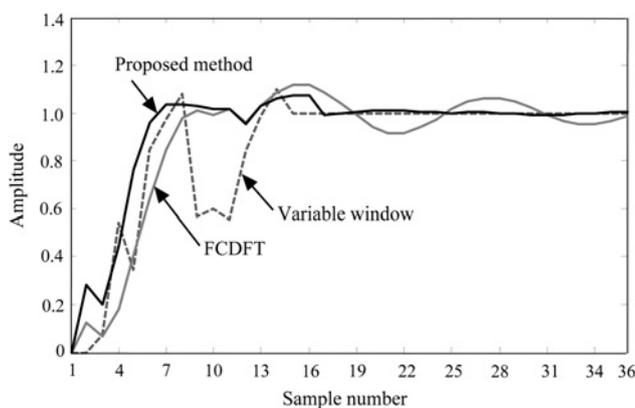
Fig. 6 Estimated phasor amplitude using the proposed, FCDFT and variable-window algorithms, case III
