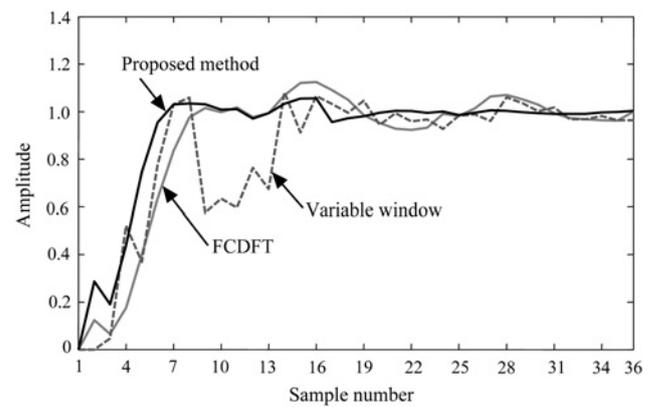
Fig. 7 Estimated phasor amplitude using the proposed, FCDFT and variable-window algorithms for a power frequency drift, case IV
