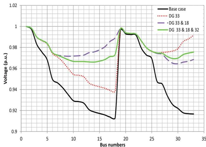
Fig. 7. Voltage profile for different placement scenarios (PL = 40%).
