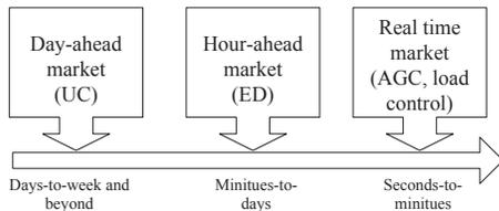
Fig. 1. Timeframe for power system operation.
