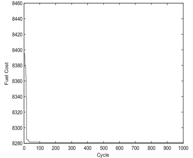
**Fig. 5.** Convergence characteristic of 3-generator system for 850 MW with considering valve point loading effect.
