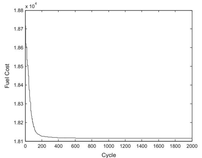
**Fig. 7.** Convergence characteristic of 13-generator system for 1800 MW by considering valve point loading effect.
