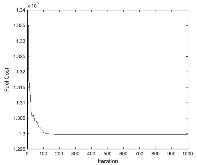
Fig. 9. Convergence characteristic of 40-generator system for 10,500 MW by considering valve point loading effect.
