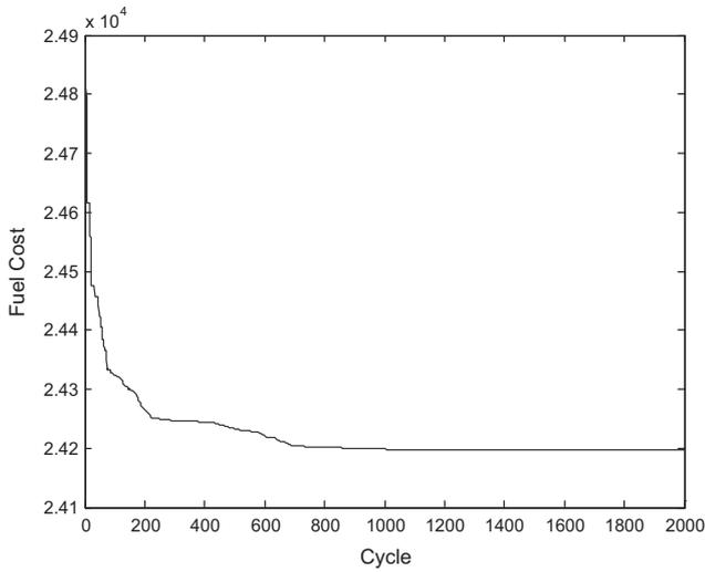
Fig. 8. Convergence characteristic of 13-generator system for 2520 MW by considering valve point loading effect.
