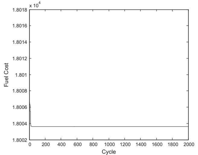
**Fig. 6.** Convergence characteristic of 13-generator system for 1800 MW.
