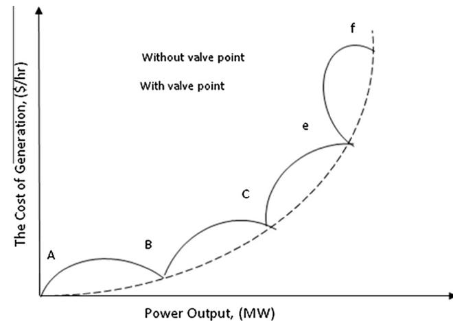
Fig. 1. Input-output curve with valve-point loading. a, b, c, d, e—valve points.
