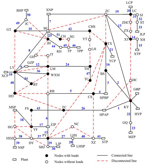
Fig. 3. The destination skeleton network for a part of the Guangdong power grid in China.
