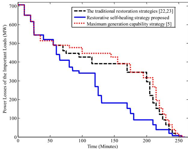
Fig. 4. Comparisons of power losses of the important loads at different time periods for Guangdong power system.
