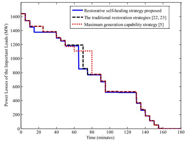
Fig. 2. Comparisons of power losses of the important loads at different time periods for the New England power system.
