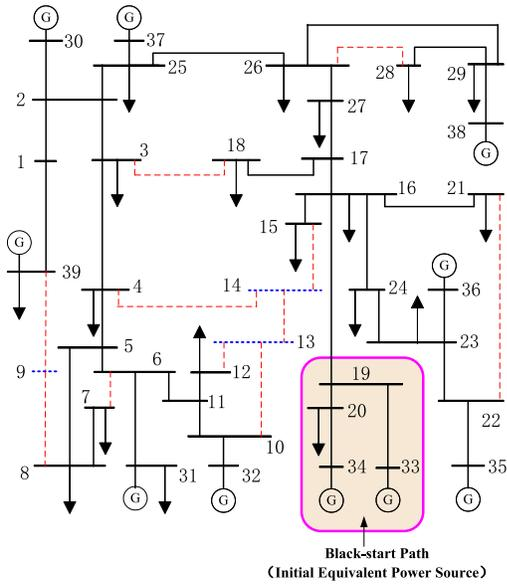
Fig. 1. The destination skeleton network in the network reconfiguration of the New England power system.
