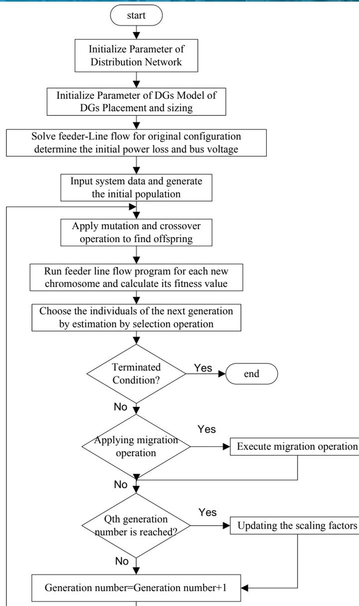
**Fig3: computational process of the VSHDE for solving network reconfiguration of distribution systems and DG placement**
