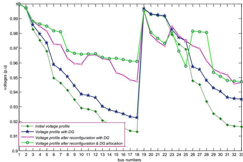
Fig 6. Comparison of voltage profiles of 33-bus distribution network
