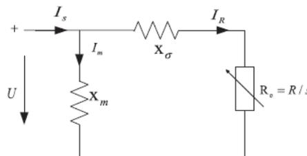
Fig. ۲. The approximate model of asynchronous generator.
