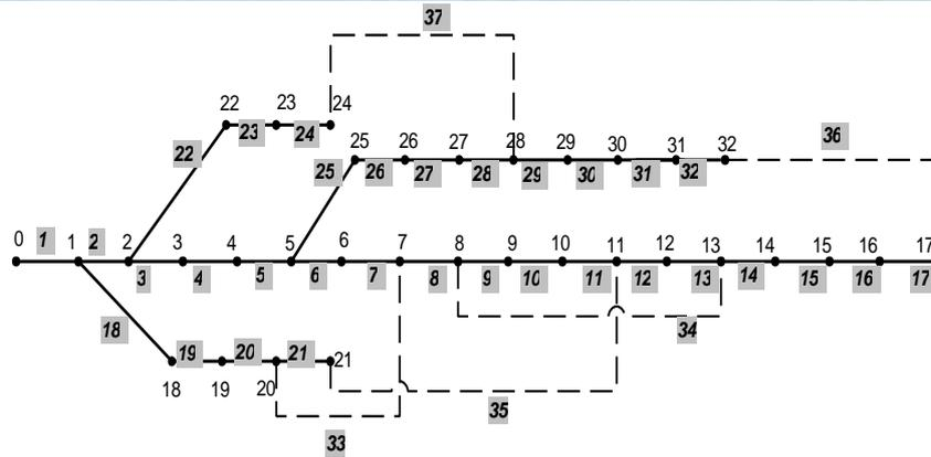
Fig ۶. Single Line diagram of ۳۳-bus radial system
