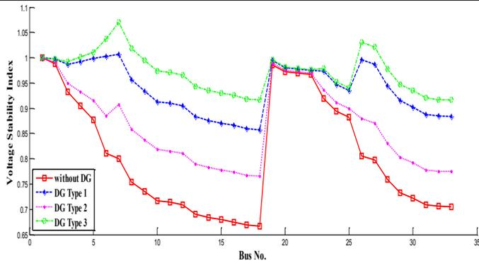
Fig. 8. Voltage stability for 33 bus test system (Case 2)
