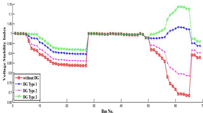
Fig. 10. Voltage stability for 69 bus test system (Case 2)
