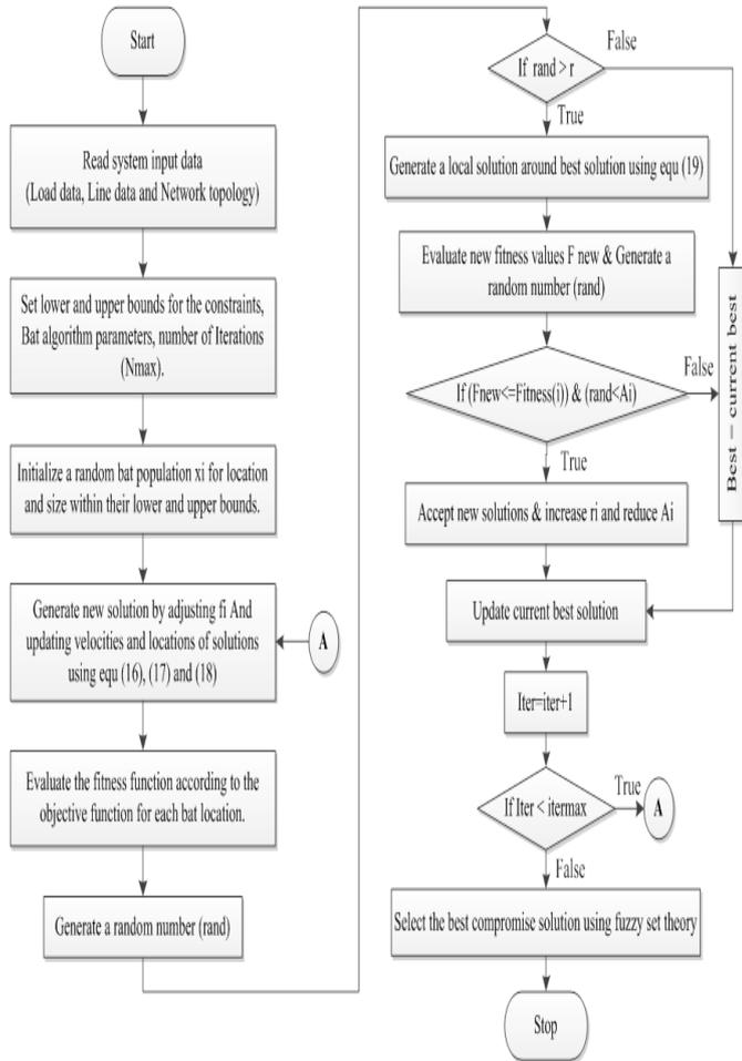
Fig. 2. BA flowchart for DG unit placement and sizing.
