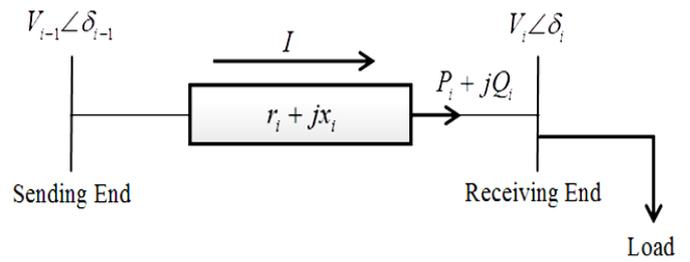
Fig. 1. A two-bus system one line diagrams.
