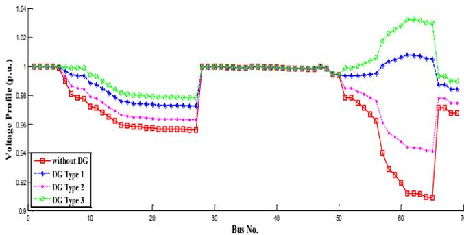
Fig. 9. Voltage profile for 69 bus test system (Case 2)
