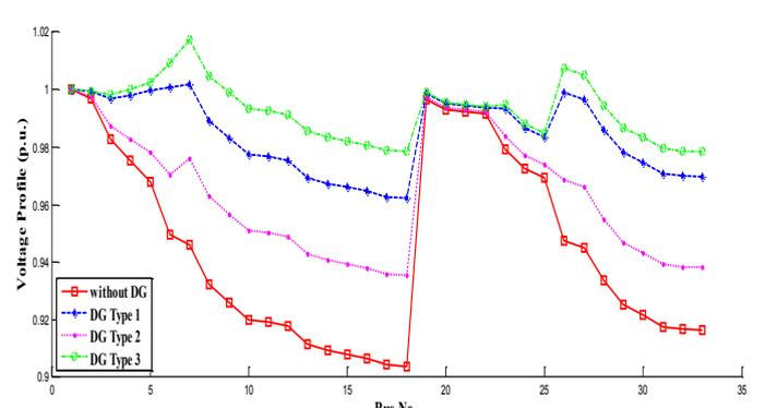
Fig. 7. Voltage profile for 33 bus test system (Case 2)
