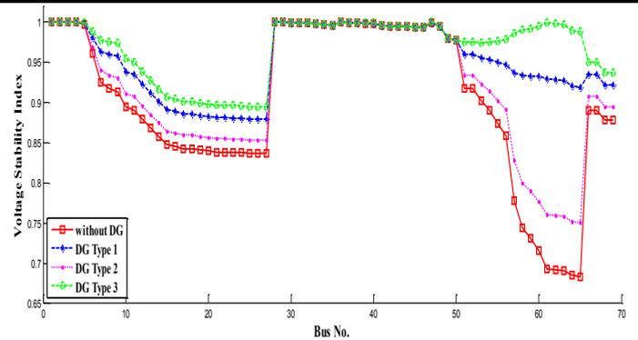
Fig. 6. Voltage stability for 69 bus test system (Case 1)
