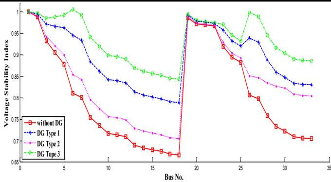
Fig. 4. Voltage stability for 33 bus test system (Case 1)
