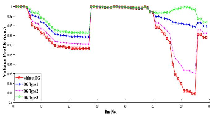
Fig. 5. Voltage profile for 69 bus test system (Case 1)
