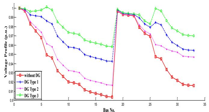
Fig. 3. Voltage profile for 33 bus test system (Case 1)
