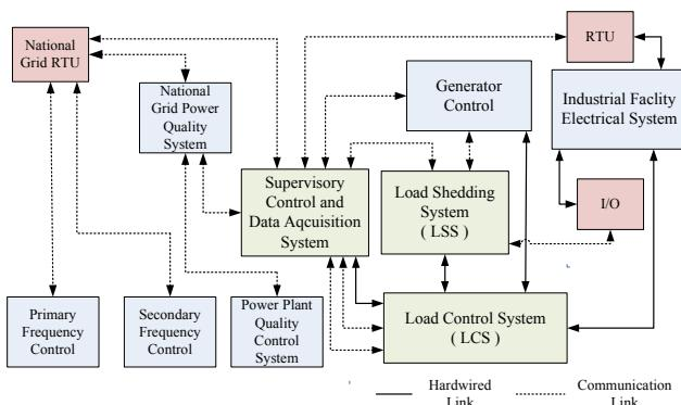
**Fig.3.** General communication interface topology of intelligent supervise, control and monitoring of industrial facility electrical system.
