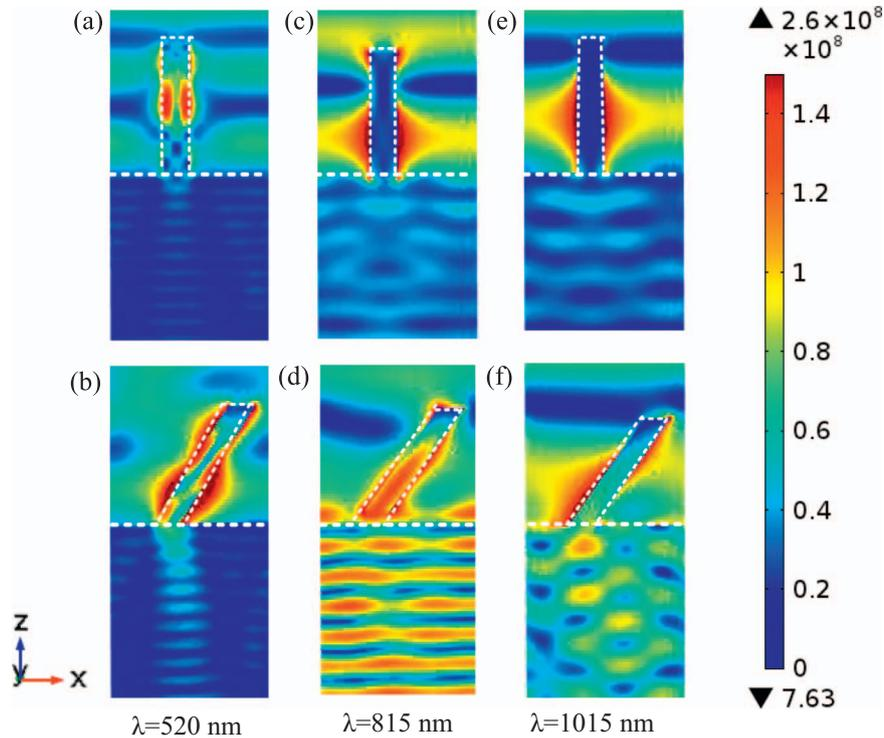
**Fig. 3.** The intensity distribution of the time-averaged TM polarized electric field at different wavelengths within the VNW ((a),(c),(e)), and the INW with  $\theta=35.4^\circ$ ((b),(d),(f)). The structures are roughly sketched by the dotted line.
