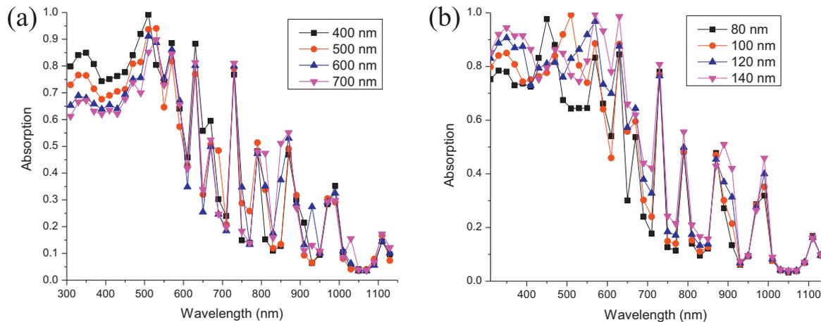
**Fig. 5.** Absorption of the INW with different periods, the diameter  $D$  is fixed at 100 nm (a), absorption of the INW with different diameters, the period  $P$  is fixed at 400 nm.
