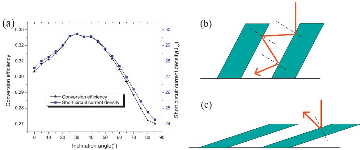
**Fig. 4.** The short circuit current density and conversion efficiency of INW with different inclination angles. The diameter and pitch are fixed at 100 nm and 600 nm respectively (a).The optical path in the INW of small (b) and large inclination angles (c).
