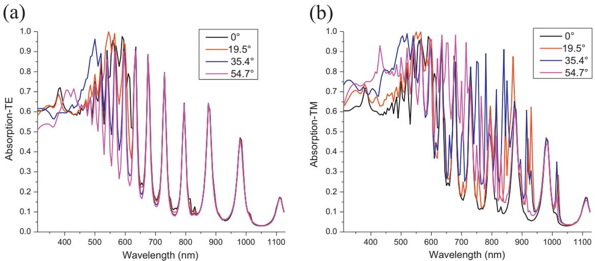
**Fig. 2.** Absorption of NW with four different inclination angles (vertical, < 110 >, < 111 > and < 112 >-oriented) as a function of wavelength, TE (a) and TM (b).
