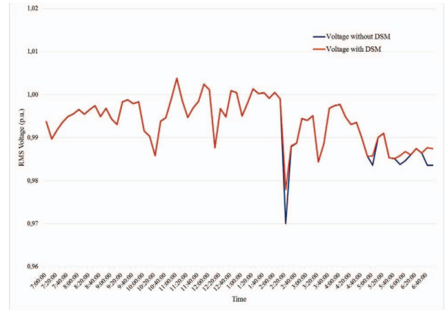
Fig. 4. Voltage at the bus 10 for simulations with and without DSM in Case study A
