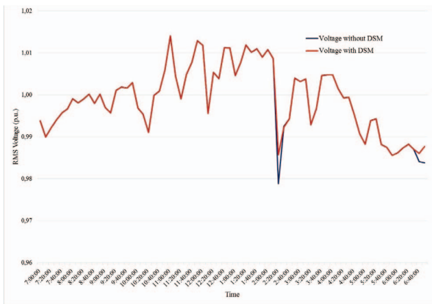
Fig. 7. Voltage at the bus 10 for simulations with and without DSM in Case study B
