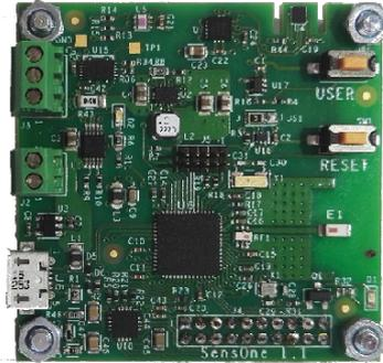
Figure 3: Base board for *NGS-PlantOne* monitoring nodes.
