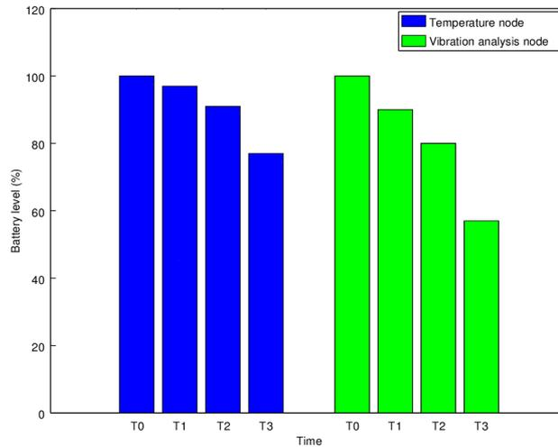
Figure 9: Average battery level for temperature and vibration analysis nodes.
