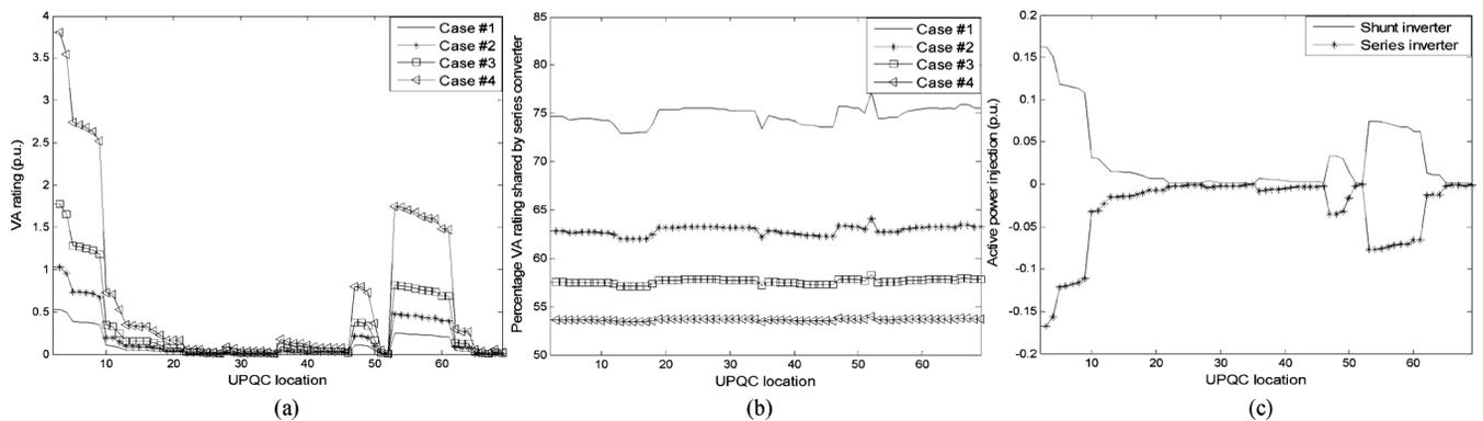
Fig. 5. UPQC-SPAC allocation at different nodes of the 69-node system: (a) VA rating, (b) percentage of VA shared by the series inverter, and (c) active power injection of series and shunt inverters.
