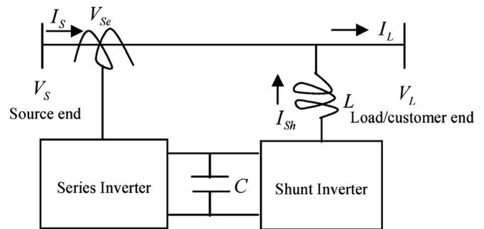
Fig. 1. Schematic of the UPQC.
