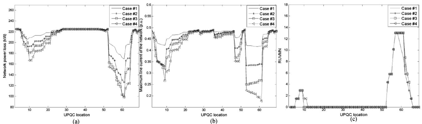
Fig. 7. Impact of UPQC-SPAC allocation at different nodes of the 69-node distribution system in view of: (a) network power loss, (b) the maximum line current of the network, and (c) RUVMN.
