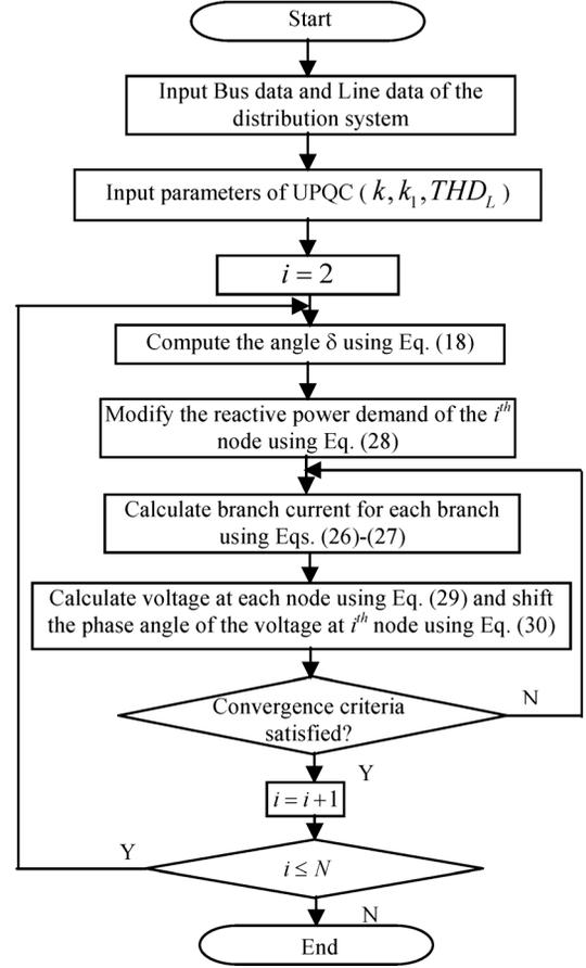
Fig. 3. Flowchart of the load-flow algorithm incorporating the UPQC-SPAC model ( $N$  = total number of nodes).
