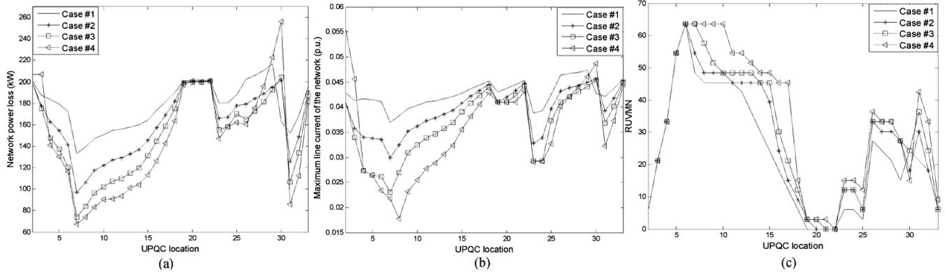
Fig. 6. Impact of UPQC-SPAC allocation at different nodes of the 33-node distribution system in view of: (a) network power loss, (b) the maximum line current of the network, and (c) RUVMN.
