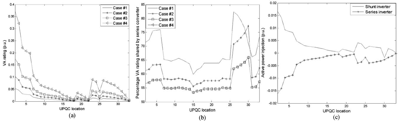
Fig. 4. UPQC-SPAC allocation at different nodes of the 33-node system: (a) VA rating, (b) percentage of VA shared by the series inverter, and (c) active power injection of series and shunt inverters.
