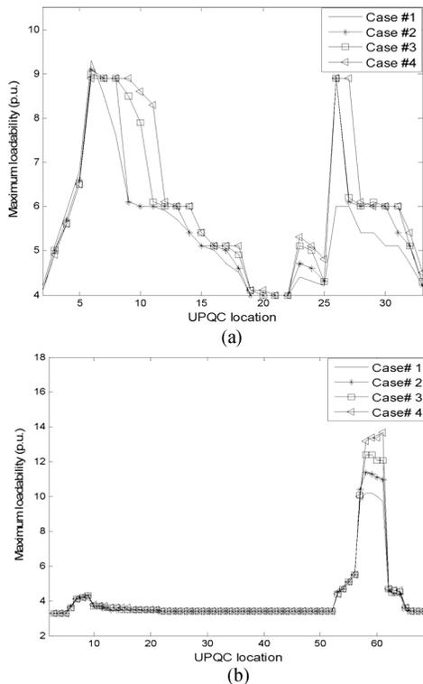
Fig. 10. Maximum loadability of the network due to UPQC-SPAC allocation at different nodes studied on the: (a) 33-node and (b) 69-node systems.
