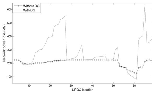
Fig. 11. Network power loss of the 69-node system with combined DG and UPQC-SPAC allocations.
