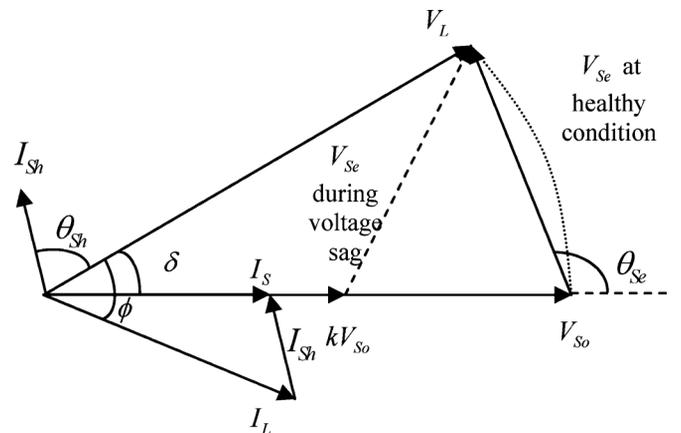
Fig. 2. Phasor diagram of shunt and series compensations of UPQC-SPAC at the normal/healthy voltage condition and during voltage sag.
