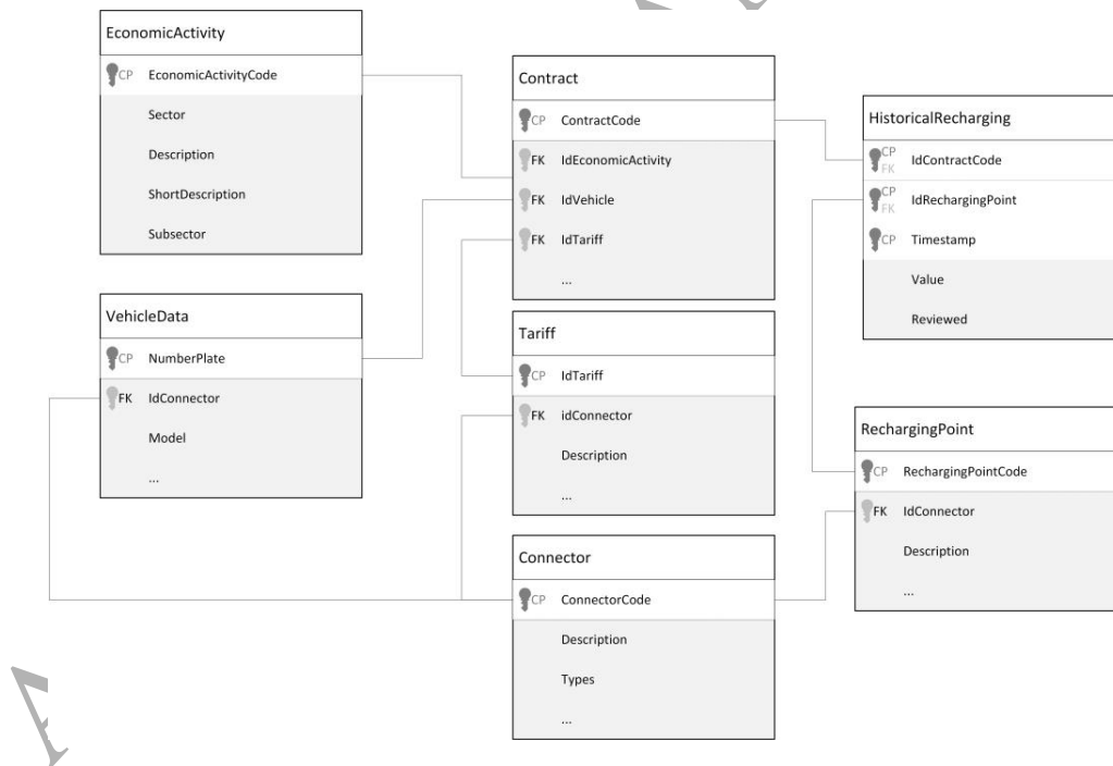
Fig. 4. UML Diagram for Source B.
