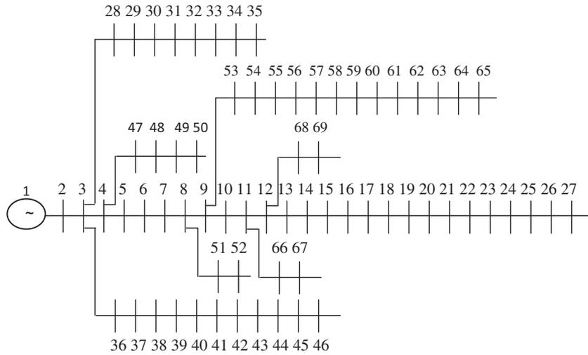
Fig. 9. Line diagram of the 69 bus system.
