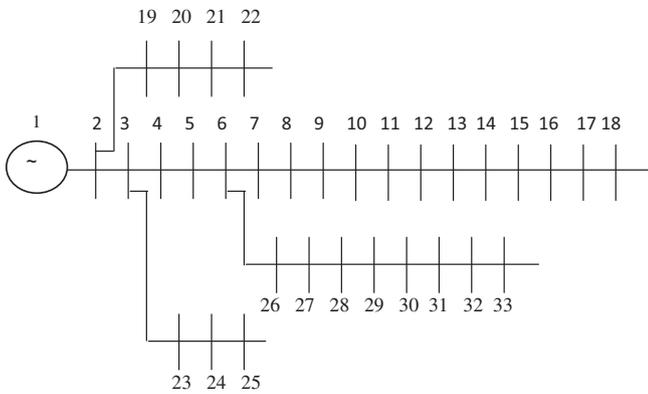
Fig. 6. The schematic diagram of the 33 bus system.
