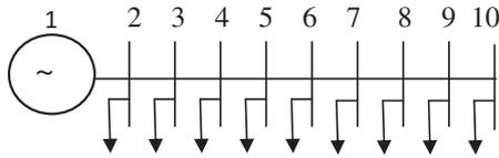
**Fig. 3.** The schematic diagram of the 10 bus system.
