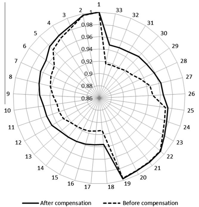
**Fig. 8.** The effect of compensated devices on voltages of 33 bus system.
