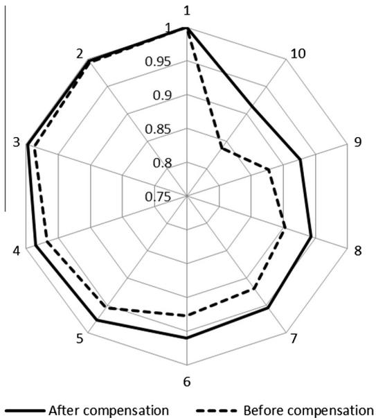
Fig. 5. The effect of compensated devices on voltages of 10 bus system.
