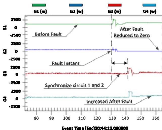
Fig. 11. The real power of each generator before and after fault at section 13.
