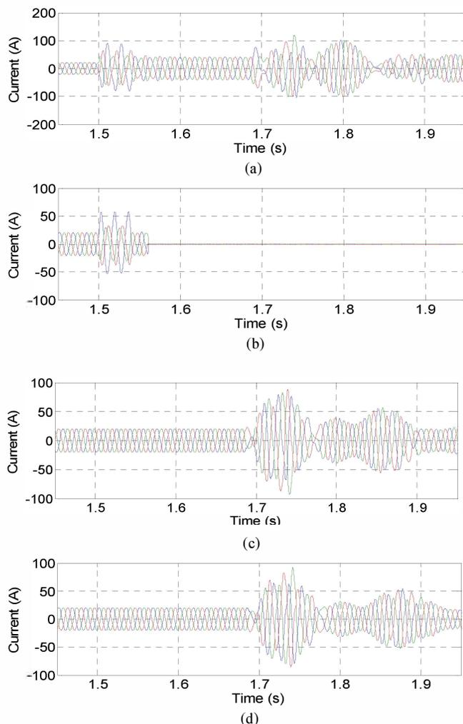
Fig. 6. The three phase current of DGs during single line to ground fault in the middle of section 13. (a) Current of DG1, (b) Current of DG2, (c) Current of DG3, (d) Current of DG4.
