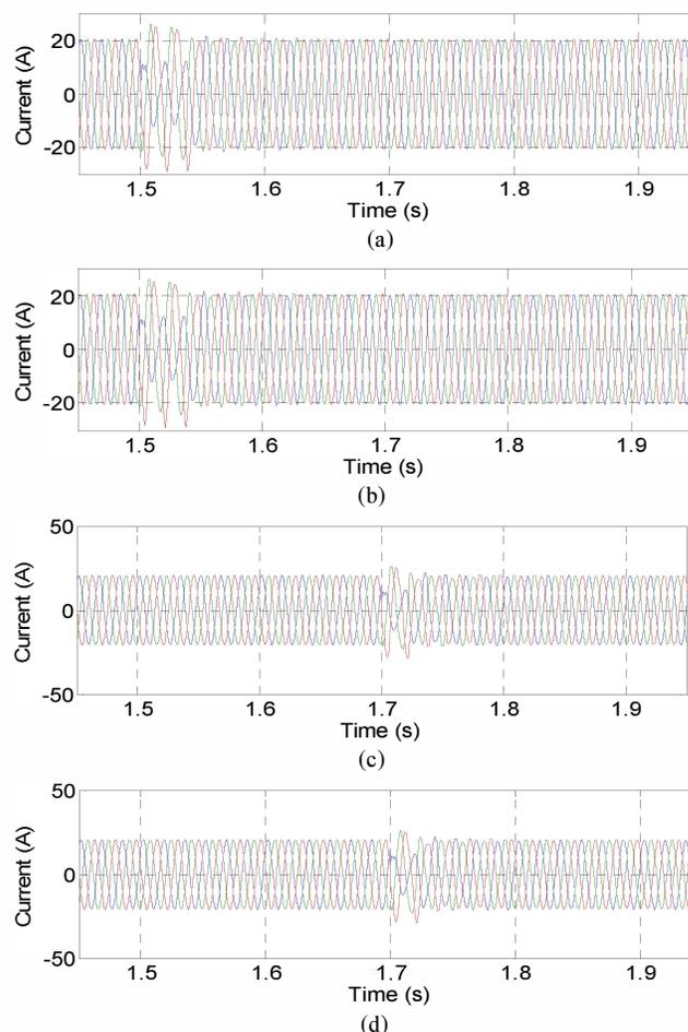
Fig. 7. The three phase current of the loads during single line to ground fault in the middle of section 13
