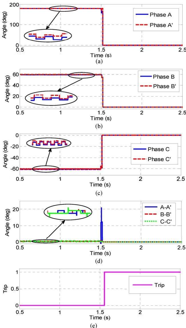
Fig. 2. Phase angles of starting and ending sides during single line to ground fault on phase A in the middle of section 13. (a) Angles of phases A, A', (b) Angles of phases B, B'. (c) Angles of phases C, C', (d) Deviation angles for phases A, B and C, (e) Tripping signal.
