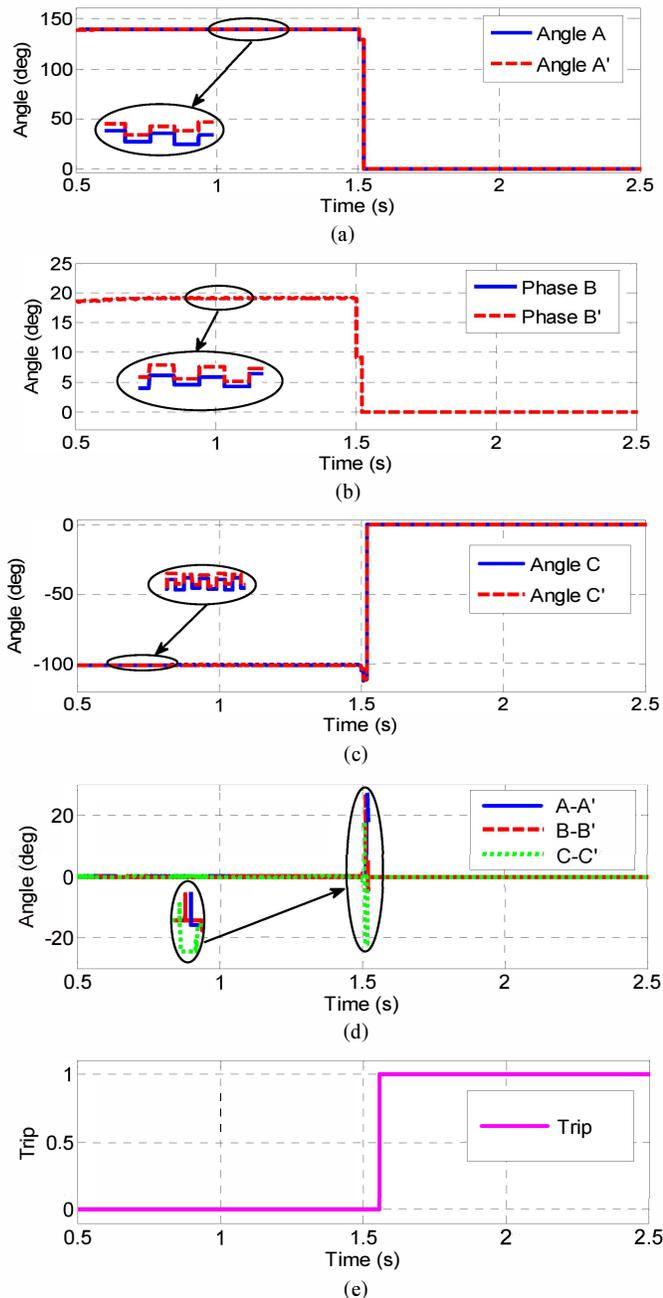
Fig. 4. Phase angles of starting and ending sides during three phase to ground fault in the middle of section 12. (a) Angles of phases A, A', (b) Angles of phases B, B', (c) Angles of phases C, C' (d) Deviation angles for phases A, B and C, (e) Tripping signal.
