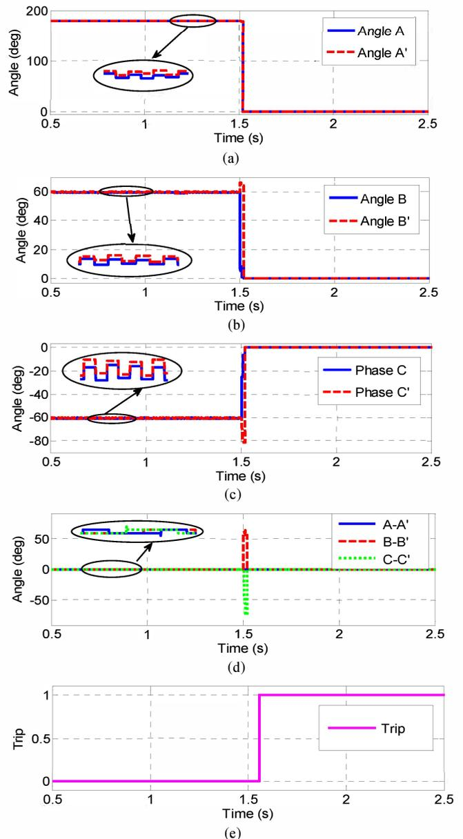
Fig. 3. Phase angles of starting and ending sides during double line to ground fault on phases B&C in the middle of section 13. (a) Angles of phases A, A', (b) Angles of phases B, B'. (c) Angles of phases C, C', (d) Deviation angles for phases A, B and C, (e) Tripping signal.
