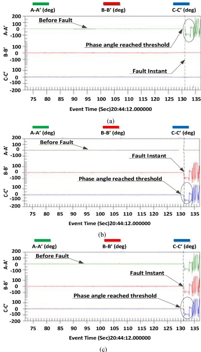
Fig. 10. Phase angle difference of starting and ending sides at section 13 during. (a) Single line to ground fault, (b) Double line to ground fault. (c) Three phase to ground fault.
