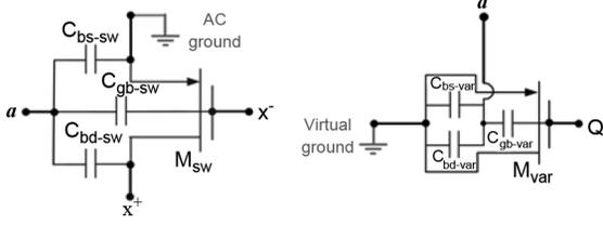
Fig. 2. Intrinsic capacitances that play the role of coupling elements.
