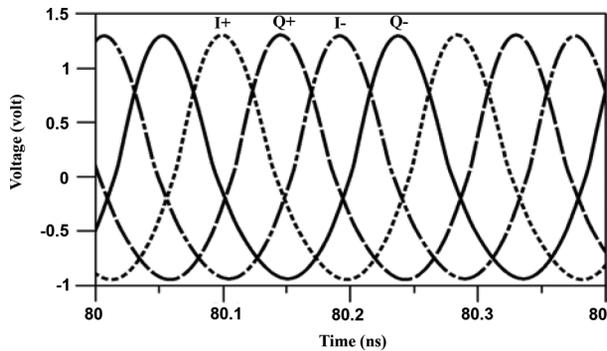
Fig. 3. Output waveforms of the proposed QVCO.
