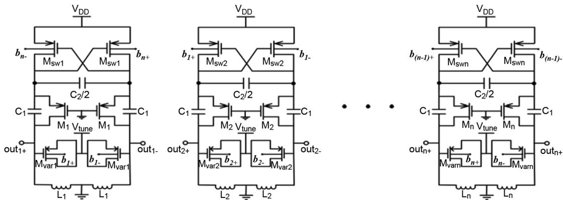
Fig. 6. Proposed multiphase VCO:  $N - 1$  core VCOs are coupled to each other in an in-phase manner and the  $N$ th VCO is coupled to the first VCO in an anti-phase manner through the bulks of the core transistors.
