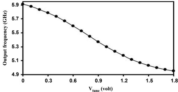
Fig. 4. Simulated frequency tuning range of the proposed QVCO.
