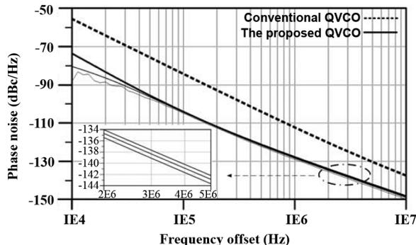
Fig. 5. Simulated phase noise of the proposed QVCO (for different coupling factors) and that of P-QVCO with coupling technique proposed in [11].
