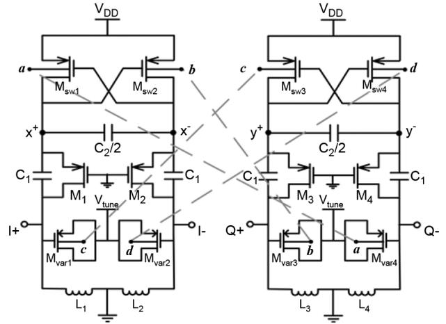
Fig. 1. Schematic of the proposed quadrature VCO.
