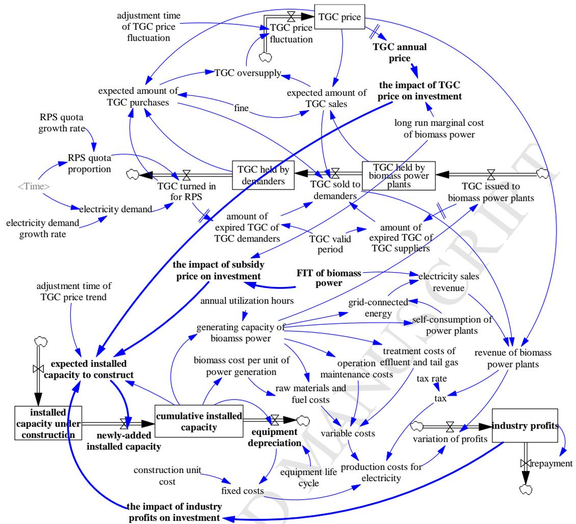
Figure 5 The flow graph of biomass power industry development under RPS scheme
