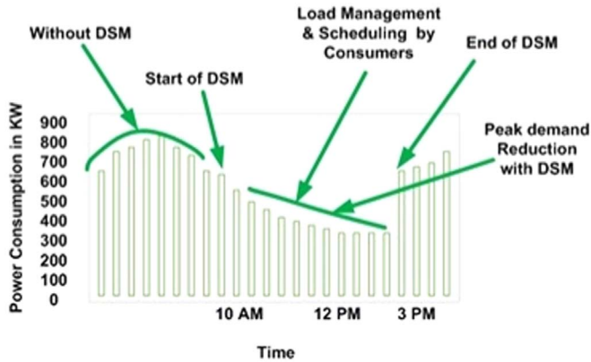
Fig. 5. Load management and reduction of peak stress on electric grid by DSM [61].
