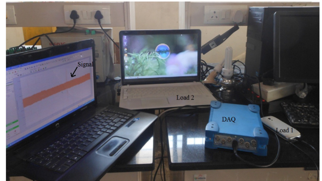
Fig. 7. Test setup for acquiring transient signal.
