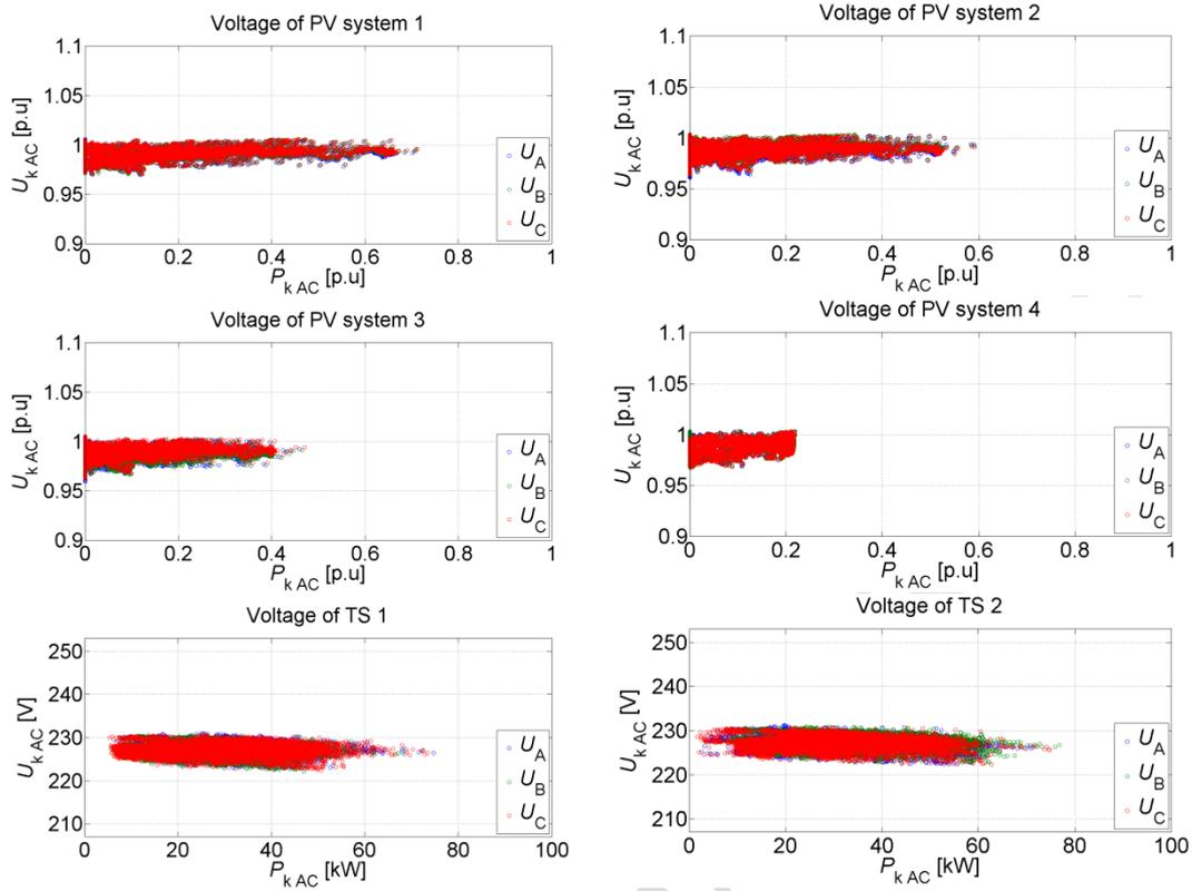
Figure 4: RMS value of output voltage  $U_{AC}$ , measured during tests, given as a function of output power  $P_{AC}$ .
