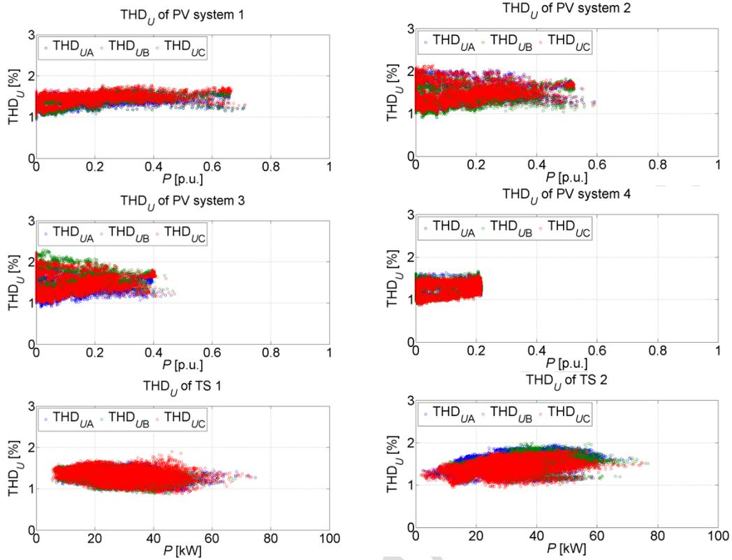
Figure 7: Voltage THD for fundamental frequency 50Hz and 40 higher order harmonic components, given as a function of output power  $P_{AC}$ .
