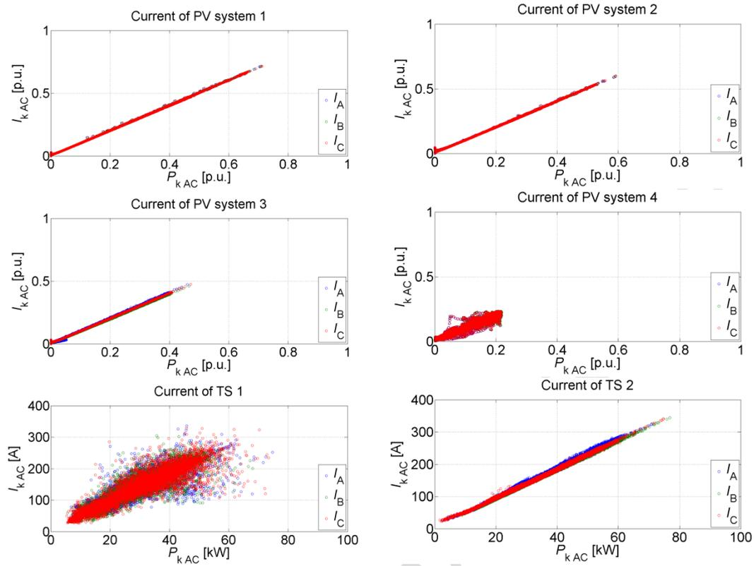
Figure 5: RMS value of output current  $I_{AC}$ , measured during tests, given as a function of output power  $P_{AC}$ .
