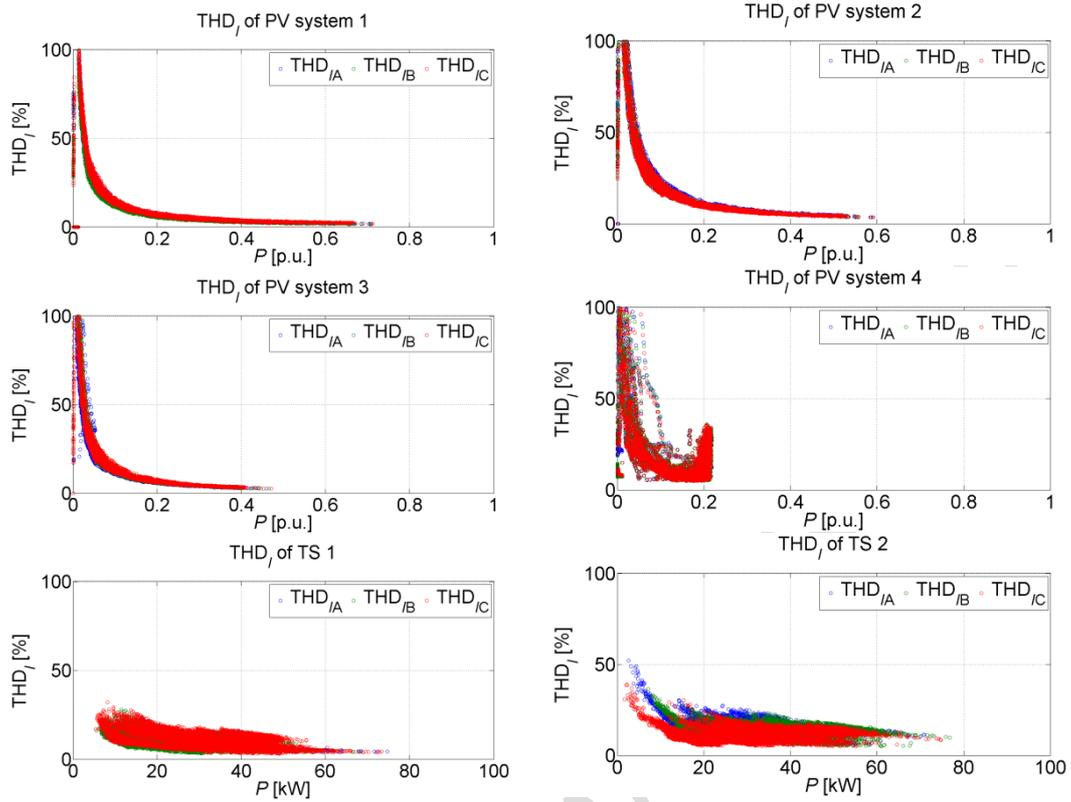
Figure 8: Current THD for fundamental frequency 50Hz and 40 higher order harmonic components, given as a function of output power  $P_{AC}$ .
