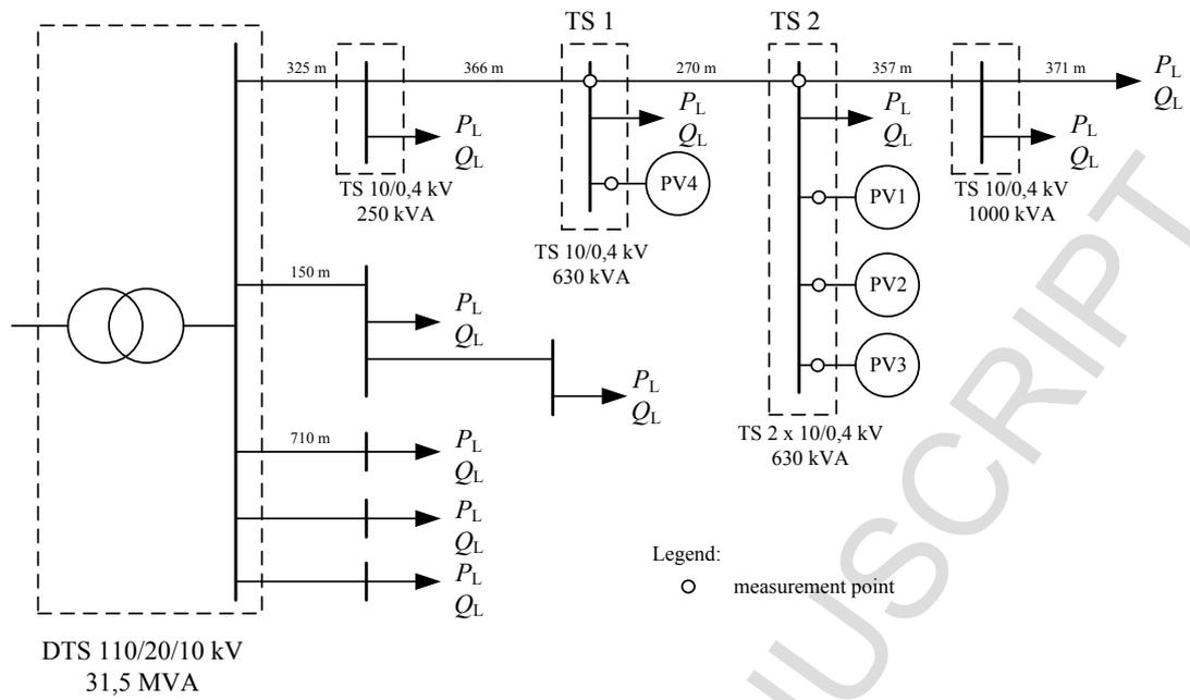
Figure 3: Discussed low voltage network with installed photovoltaic systems.
