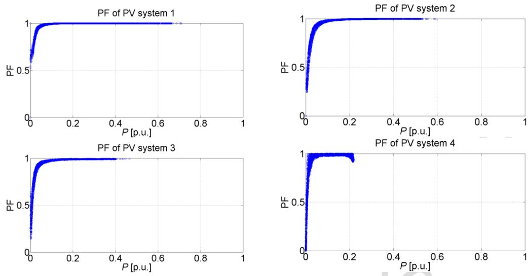
**Figure 9: Power factor  $PF$  measured during tests, given as a function of output power  $P_{AC}$ .**
