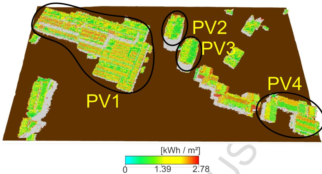
Figure 10: Estimated photovoltaic potential of the PV1, PV2, PV3, and PV4 systems.
