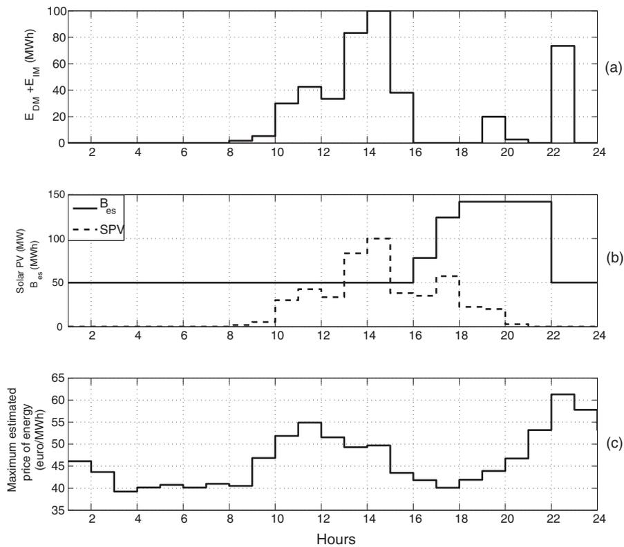
**Fig. 14.** Day type: cloudy day. Scheduling results. Date 04/25/2015. (a) Daily and intraday markets energy  $E_{DM} + E_{IM}$ . (b) Solar PV Generation and energy stored in the battery  $B_{es}$ . (c) Maximum estimated price of energy.
