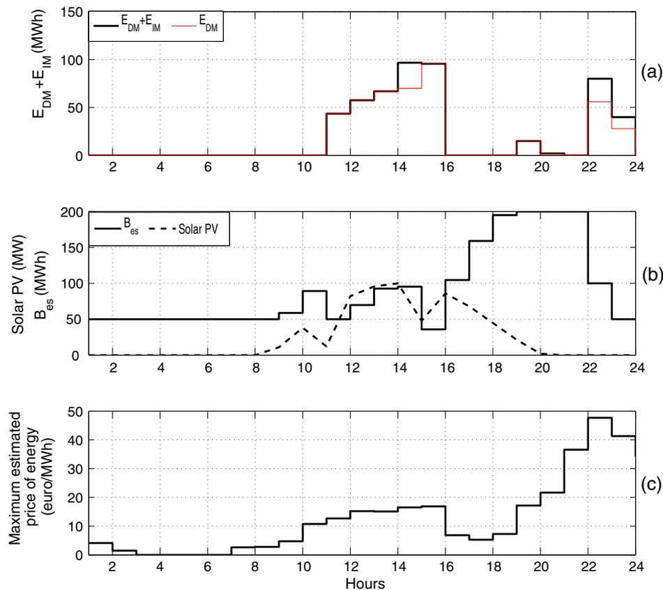
Fig. 11. Day type: clear day with unexpected clouds. Scheduling results:  $MPC_{IMs1}$ . Date 04/05/2015. (a) Daily and intraday markets energy  $E_{DM} + E_{IM}$ . (b) Solar PV Generation and energy stored in the battery  $B_{es}$ . (c) Maximum estimated price of energy.
