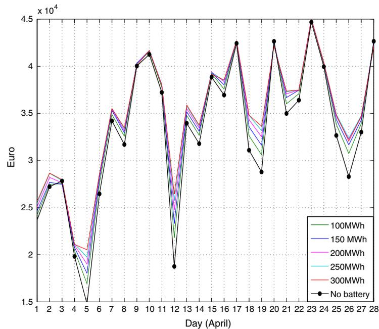
Fig. 17. Profits obtained through the use of the scheduling algorithm with different battery capacities compared to a plant without energy storage. April 2015.
