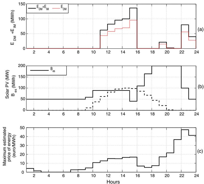
**Fig. 9.** Day type: clear day. Scheduling results. Date 04/05/2015. (a) Daily and intraday markets energy  $E_{DM} + EP_{IM}$ . (b) Solar PV Generation and energy stored in the battery  $B_{es}$ . (c) Maximum estimated price of energy.
