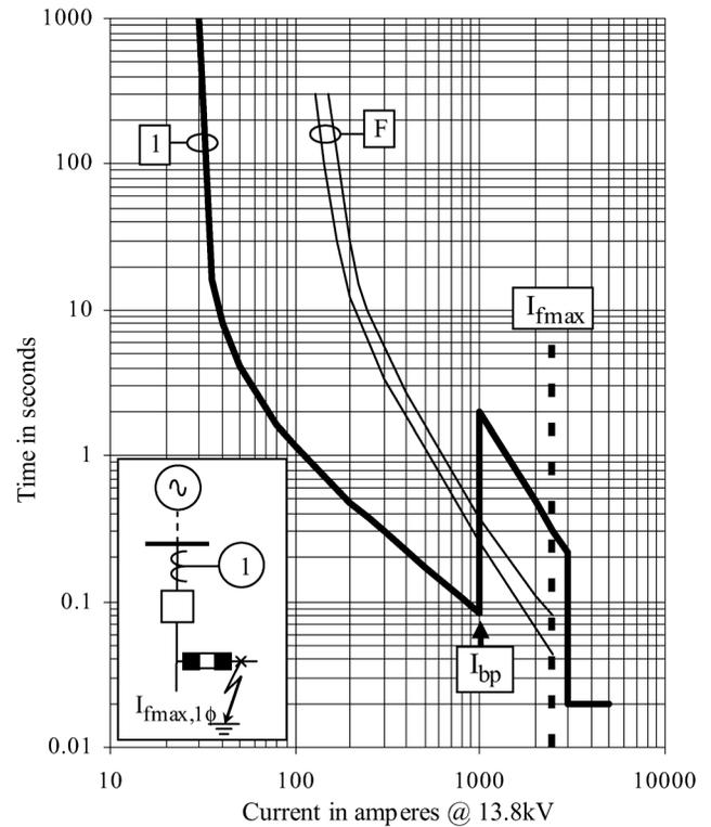
Fig. 4. Nontraditional coordination of the ground overcurrent function with downstream fuses. Case: with recloser function (first trips).
