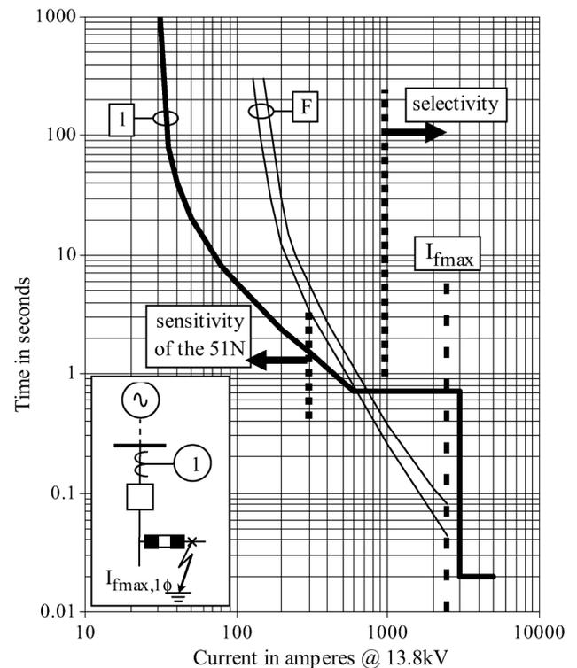
Fig. 2. Traditional coordination of the ground overcurrent function with downstream fuses. This is a good traditional solution for this case because the relay curve is limited to be inverse until  $M = 20$ .
