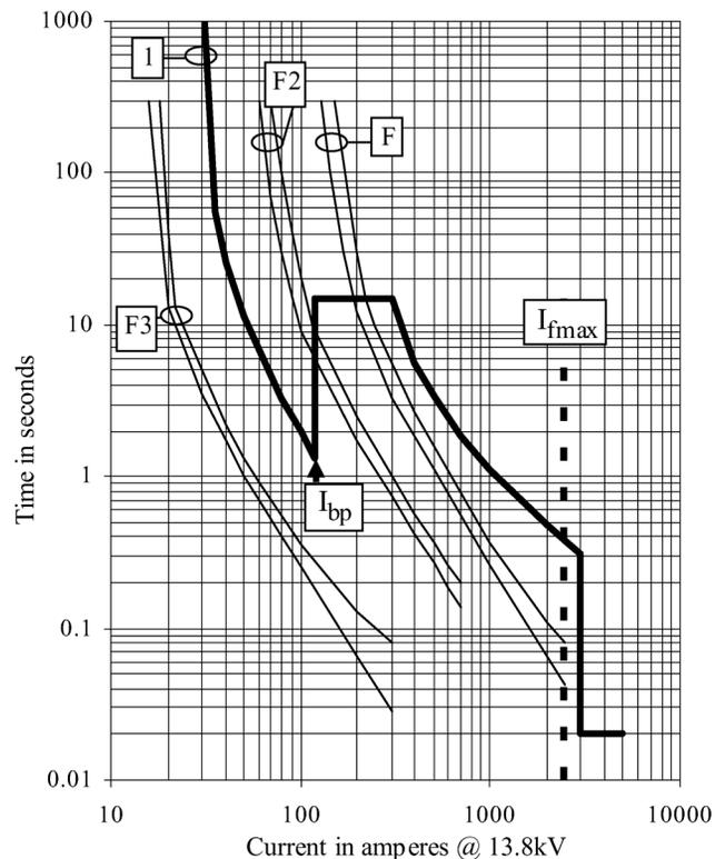
Fig. 11. Case of Fig. 3, considering three different downstream fuses and a different nontraditional curve (51N), in order to maximize selectivity.
