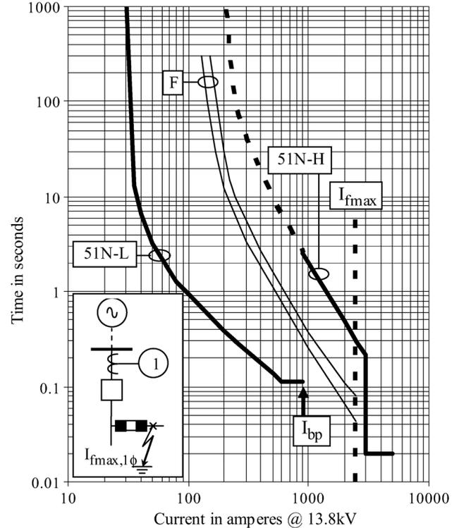
Fig. 8. Case of Fig. 4, implemented by applying logical combination of traditional curves (limits in curve shapes for  $M \geq 20$  are considered).
