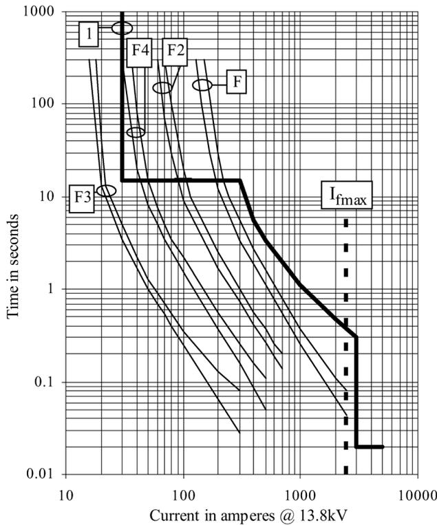
Fig. 12. Case of Fig. 3, considering four different downstream fuses, and the minimum melting current of one of them is similar to the pickup value of the nontraditional 51N function.
