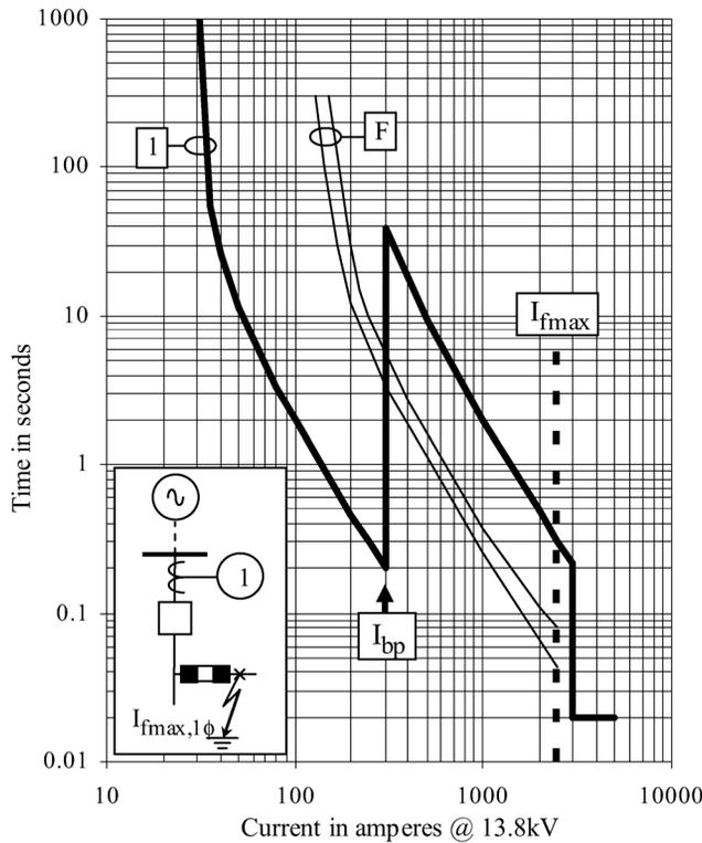
Fig. 3. Nontraditional coordination of the ground overcurrent function with downstream fuses. Case: without the recloser function.
