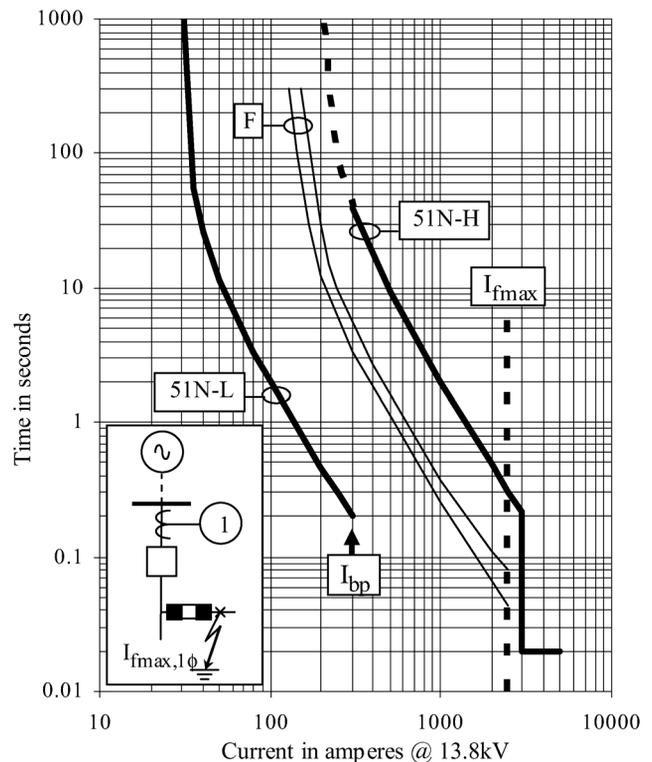
Fig. 5. Case of Fig. 3, implemented by applying a logical combination of traditional curves. (51N-L and 51N-H are 51N functions of relay 1.)
