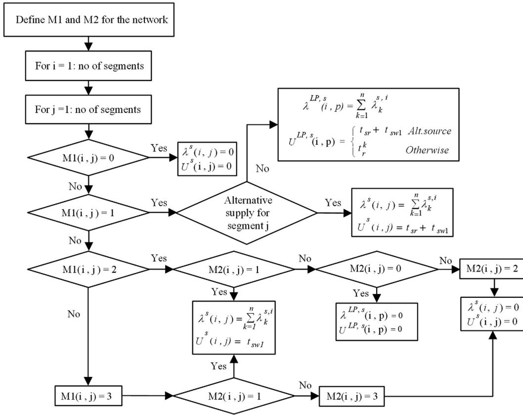
Fig. 3. Segment based failure modes and effects evaluation by looking at segments as single load points.
