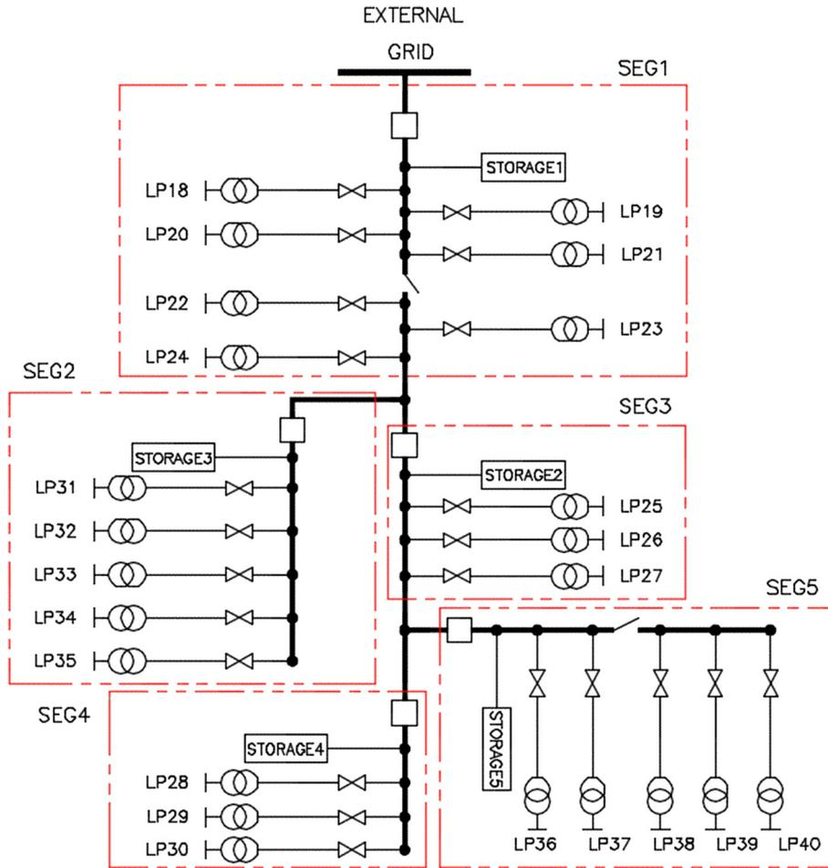
Fig. 4. Modified feeder 4 at bus 6 of the RBTS network [28].
