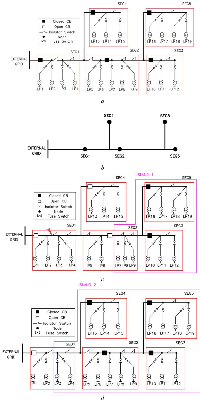
Fig. 2. Distribution network single line diagram. (a) Distribution network divided into segments. (b) Aggregated load and PV in each segment to simplify the network. (c) Island 1 formation immediately after fault occurrence in segment 1. (d) Island 2 formation after fault is isolated manually in segment 1.
