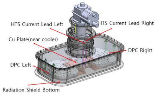
Fig. 9. Position of temperature sensor
