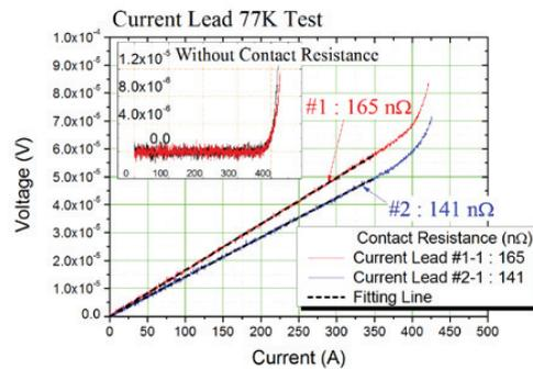
Fig. 6. Characteristics of HTS current lead at 77 K.
