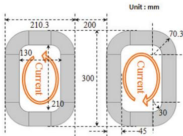
Fig. 2. Dimension of superconducting coil.
