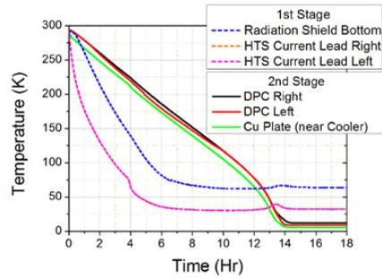
Fig. 10. Results of cooling the magnet
