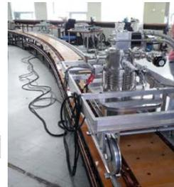
Fig. 13. Test of demo LSM system
