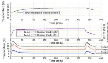
Fig. 12. Temperature variation of magnet at 130 A
