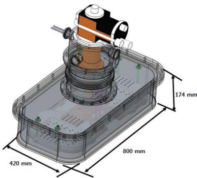
Fig. 7. Dimensions of cryostat.
