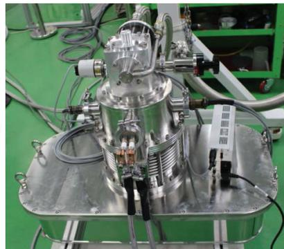
Fig. 8. Superconducting magnet system
